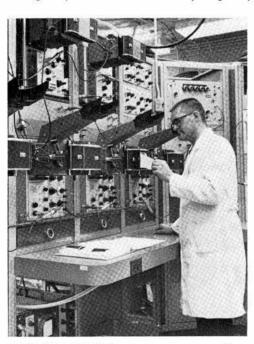
PULLING PRINTS from cameras on oscilloscopes is C. W. Huddle (5134-1). Many other diagnostic "tools" are available for high explosive tests at both firing sites.
